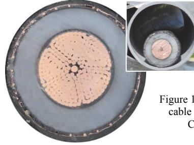
Figure 10: Indian River-Bishop 5000kcmil cable (119mm) from Prysmian Wire & Cable's Abbeville, SC factory (inset: in 8in conduit).
