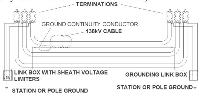
Figure 3: Single point bonding scheme used for cable projects
