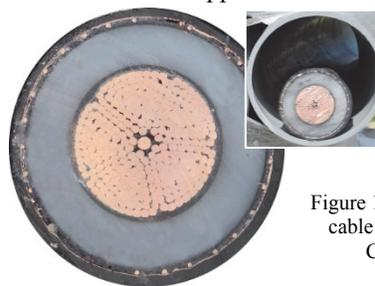
Figure 10: Indian River–Bishop 5000kcmil cable (119mm) from Prysmian Wire & Cable’s Abbeville, SC factory (inset: in 8in conduit).
