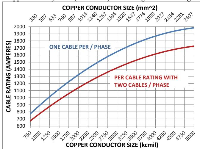
Figure 2: Variation in ampacity as a function of conductor size
